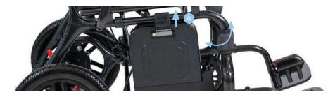
Follow the the same procedure on the left hand side to install the secondary spare battery to the chair.
