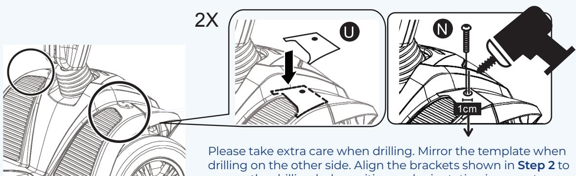
Please take extra care when drilling. Mirror the template when drilling on the other side. Align the brackets shown in **Step 2** to ensure the drilling hole position and orientation is correct.
