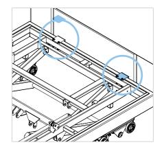
4 Fix the spacers to the bottom of the bracket once in position with 2x M6 x 20 screws.
