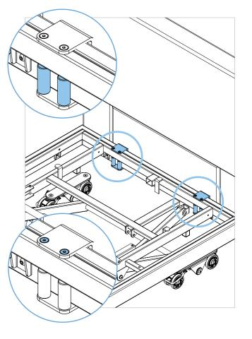
6 Position bed with 80mm spacing from the wall to give enough space for the Trendelenburg movement of the bed.
