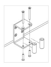
5 Align to mounting holes in frame and tighten both top and bottom bolts to secure brackets in place. Make sure the headboard is secure with minimal movement between bracket and frame.
